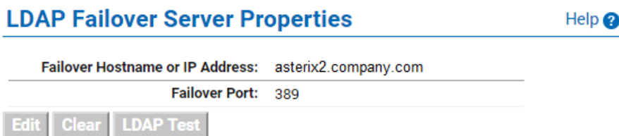
Figure 122 : LDAP Failover Server Properties
